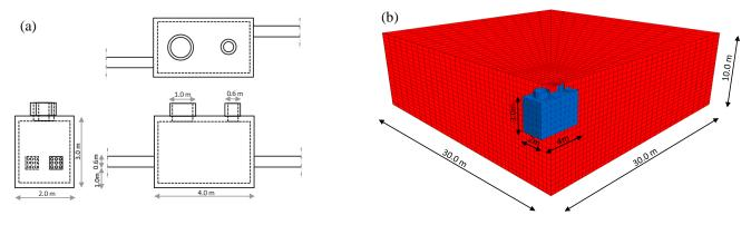
Figure 1. Numerical model: (a) Structure dimension, (b) Model layout.
