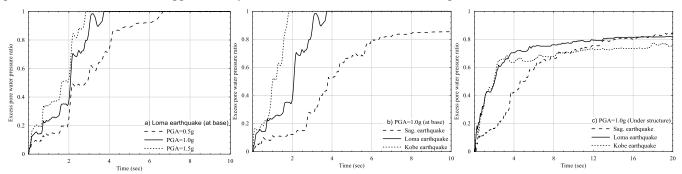
Fig. 5 Time history of liquefaction ratio: (a) at the soil base with different PGA (Loma Earthquake); (b) at the soil base with different earthquakes (PGA = 1.0g); (c) under the structure with different earthquakes (PGA = 1.0).
