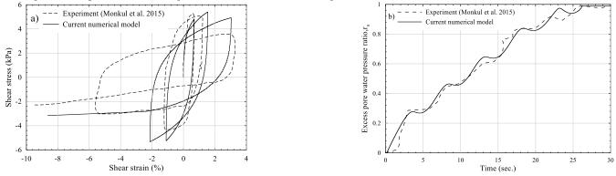
Fig. 2 Comparison between cyclic simple shear test results of Monkul et al. (2015) and current numerical simulations (a) shear stress-strain path (b) excess pore water pressure ratio ru.
