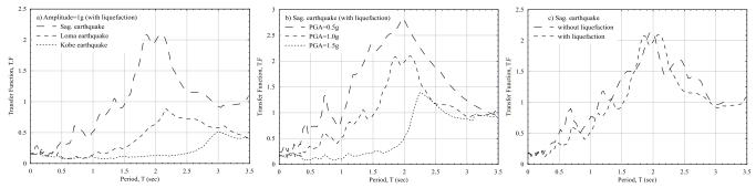
Fig. 6 Transfer Function between the output Fourier-Amplitude spectra at the surface to the input Fourier-Amplitude spectra at the base: (a) for different frequency contents; (b) for different earthquake amplitudes.
